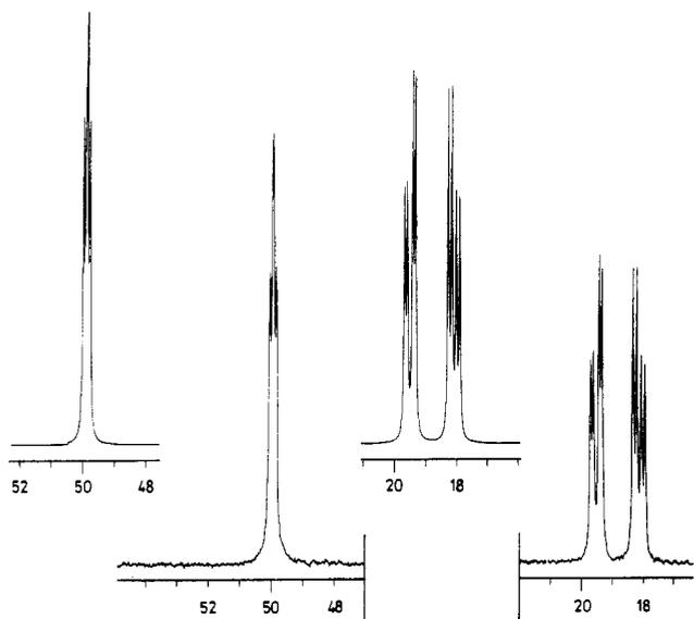
Figure 1. Experimental (lower part) and simulated (upper part) proton-decoupled  $^{31}\text{P}$  NMR spectra of  $(\text{NPCl}_2)_2\text{NP-}t\text{-C}_4\text{H}_9\text{CH(OH)CH}_3$ .
